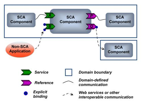
A binding specifies exactly how communication should be done between an SCA component and something else. Depending on what it's communicating with, a component might or might not have explicitly specified bindings. As the figure shows, a component that communicates with another component in the same domain, even one in another process or on another machine, need not have any explicit bindings specified. Instead, the runtime determines what bindings to use, freeing the developer from this chore.
