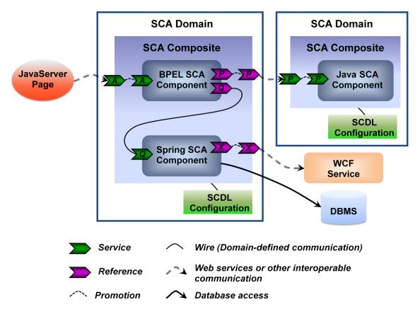
In this example, the client is a JavaServer Page. This JSP invokes service A, which is provided by an SCA component that's part of a simple composite in some SCA domain. This component is implemented in
