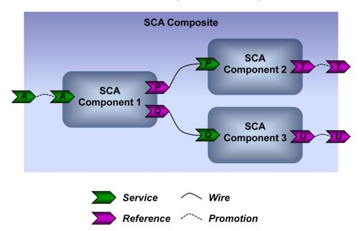
As usual, it's useful to start with a picture. The figure below shows three components, each with some combination of services and references. All three are part of the same composite.
