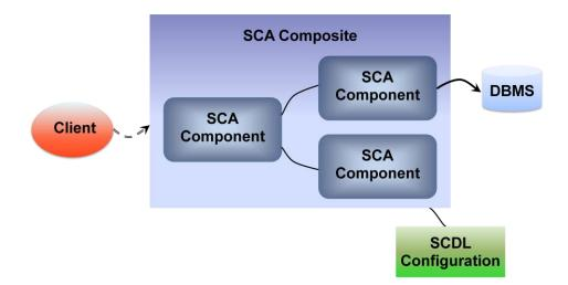
A composite is a logical construct: Its components can run in a single process on a single computer or be distributed across multiple processes on multiple computers. A complete application might be constructed from just one composite, as in the example shown here, or it could combine several different composites. The components making up each composite might all use the same technology, or they might be built using different technologies—either option is possible.
