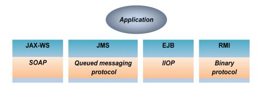
SCA takes a simpler approach. Rather than wrapping different protocols into distinct technologies with different APIs, SCA allows each remotable service and each reference to specify the protocols it supports using bindings. The programming model seen by an application remains the same regardless of which protocol is used, as the figure below illustrates.
